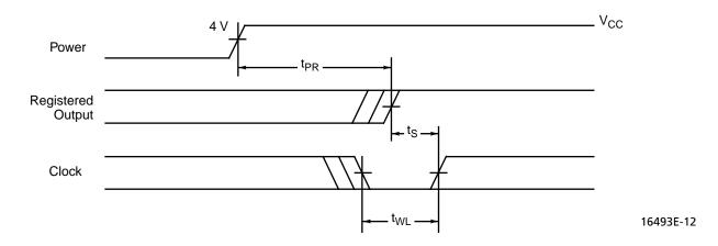
Figure 3. Power-Up Reset Waveform
